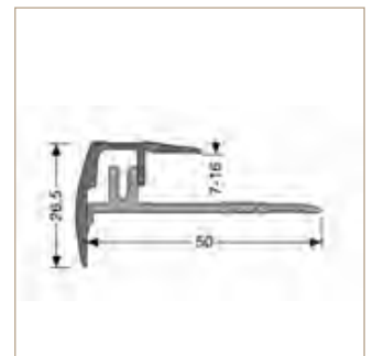
Stair edge profile PF 320 For Laminate and Parquet floors, Aluminium anodized 7–16 mm
