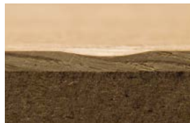
moderna parquet flooring with HDF middle layer (2.5-mm oak covering layer)
