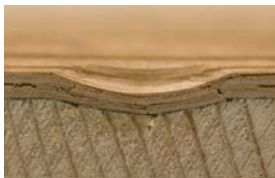
Conventional parquet flooring with spruce core (3.6-mm oak covering layer)
